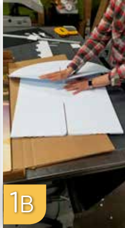
The board is stiff so you will need to use one hand to hold firmly and one to bend.
